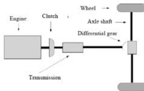
Fig. 2. Schematic diagram of the conventional driveline
