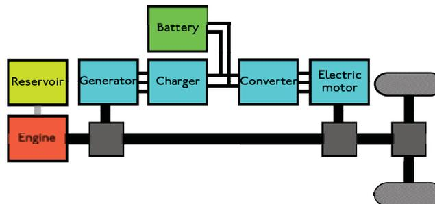
Fig. 4. Power split combined hybrid powertrain
