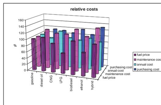
Fig. 9. Relative costs. Input cost parameters of the model were expressed as relative costs (Costs were in all cases proportioned to the cost of gasoline)
